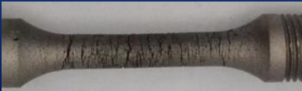
Opening of in-bulk multiple microcracks in the operated steel
