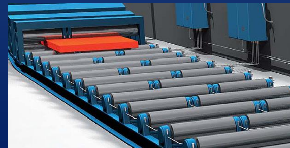
Rollers of continuous casting machine
