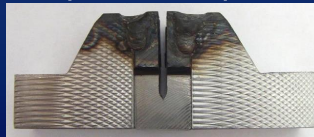
Designed short transverse V-notch specimen for impact testing
