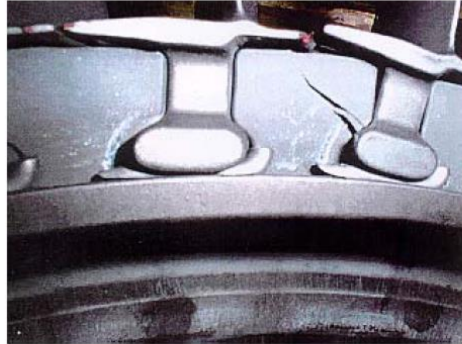
Figure-1a Bladed disk dovetail attachment region and its associated damage.
