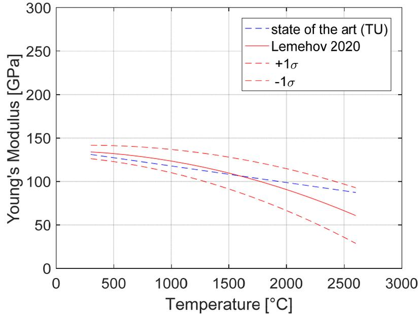
Figure 2: The standard TRANSURANUS correlation (state of the art) for Young's modulus of 30 % MOX fuel with O/M = 1.99 and porosity  $p = 0.15$ , compared to the correlation developed by S. Lemehov (including  $\pm 1\sigma$  uncertainty).
