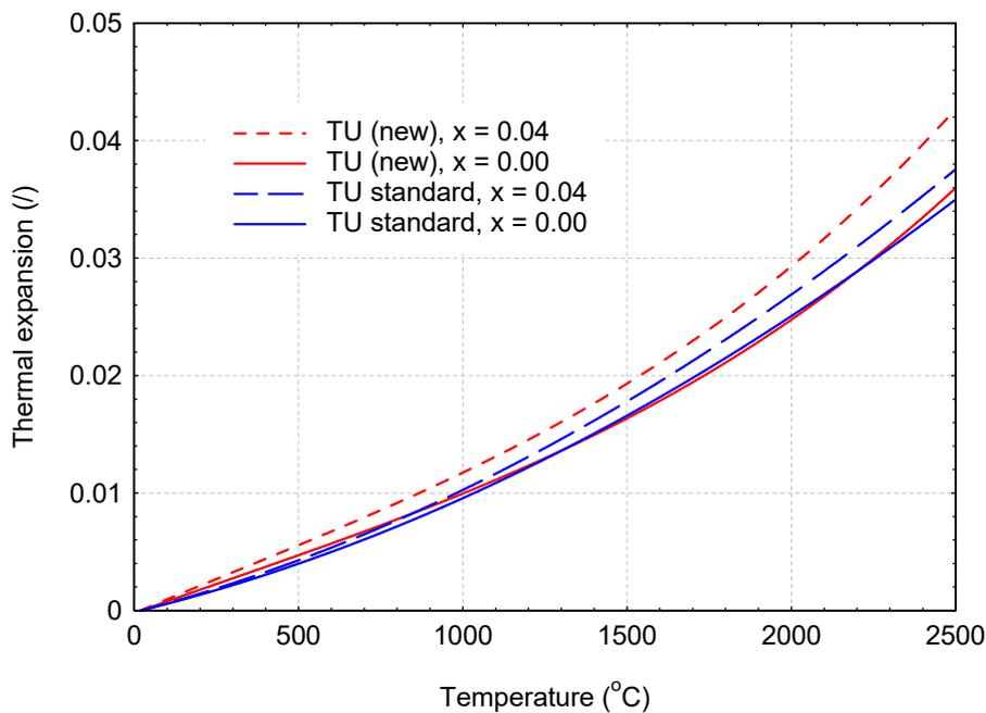
Figure 4: Comparison of the standard correlation of TRANSURANUS for the thermal expansion coefficient with the new proposed correlation developed in INSPYRE, for fresh FBR MOX fuel, as a function of the temperature (°C).
