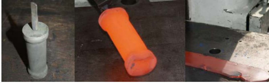
Fig. 1. Snap-shots of ODS steel fabrication via HIP (left) and HR (middle and right).
